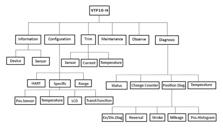
Figure 3.9 – VTP10-H programming tree.
