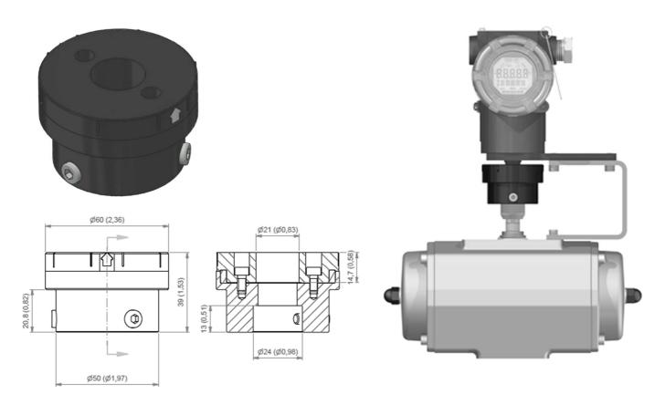
Figure 2.11 – Dimension and assembly of rotative magnet.
