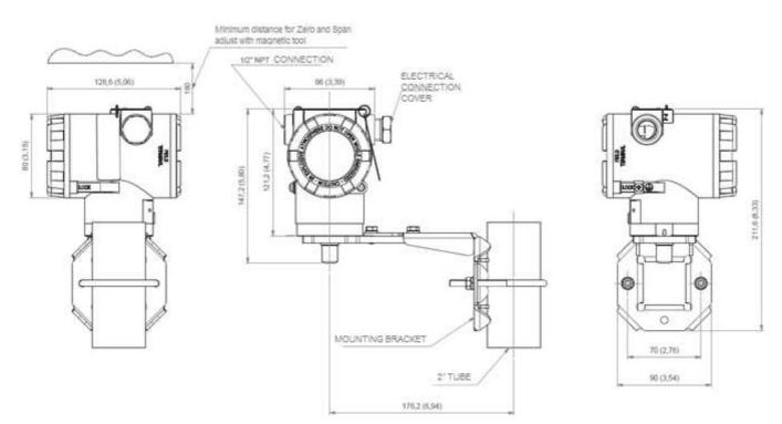
Figure 2.1 – Dimensional and mounting drawings for VTP10-H.
