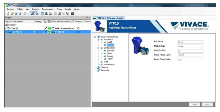
Figure 3.13 - DTM sensor configuration screen for VTP10-H.
