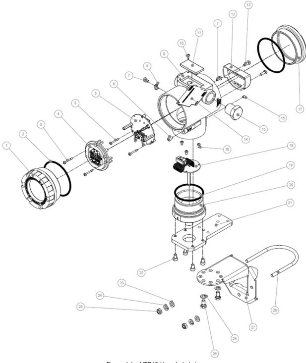
Figure 4.1 – VTP10-H exploded view.
