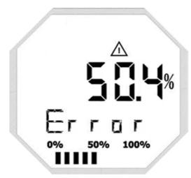
Figure 3.11 - Specific error Indication on VTP10-H.
