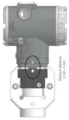
Figure 2.5 – VTP10-H assembly on rotative system.
