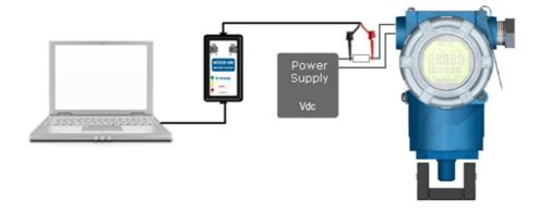
Figure 3.5 - Transmitter installation for configuration with external power supply and 250 ohms resistance.
