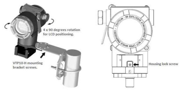
Figure 2.3 - VTP10-H bracket fixation and housing  $4 \times 90^{\circ}$  rotation.
