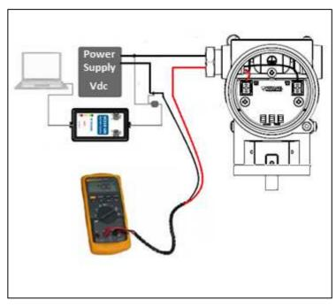
Figure 3.10 – Output current trim assembly.
