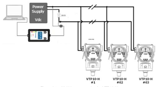
Figure 3.7 – Multidrop connection for VTP10-H.
