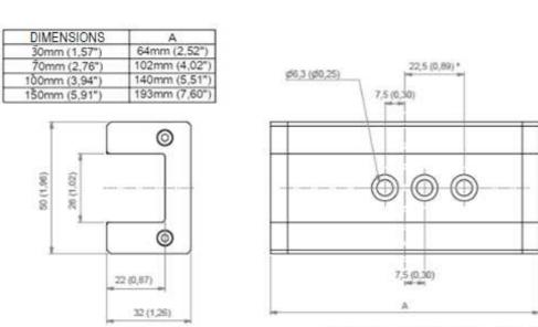
Figure 2.12 – Dimension and assembly for linear magnet models.
