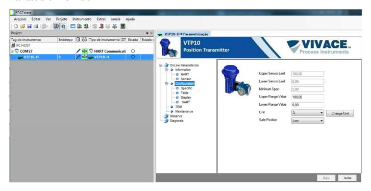
Figure 3.12 - DTM work range configuration screen for VTP10-H.
