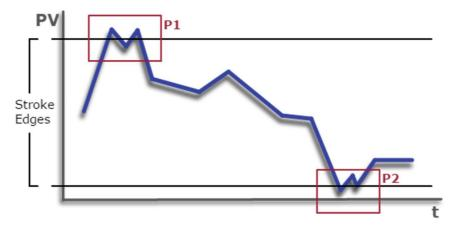
Figure 3.13 – Example of stroke occurrence on VTP10-H.
