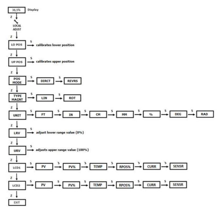
Figure 3.3 – Local adjust configuration tree.
