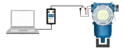
Figure 3.6 - Transmitter installation for configuration using VCI10-UH to power the device.
