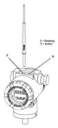
Transmitter's local configuration is executed by using Vivace's magnetic screwdriver on Z and S orifices, located at housing superior side, under identification plate. Orifice Z starts local configuration and changes the field to be configured. Orifice S is responsible for changing and saving the new value on the selected field. Saving after LCD value changing is automatic.
