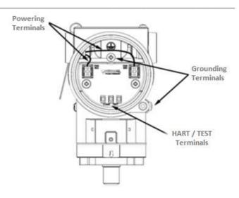
Figure 2.9 – VTP10-H connections and terminal description.
