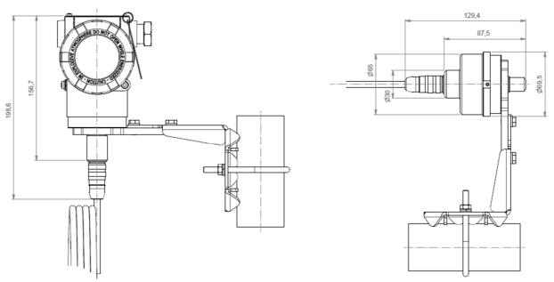
Figure 2.13 - Remote sensor dimensional drawing.
