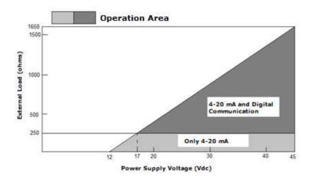
Figure 3.8 – VTP10-H load curve.
